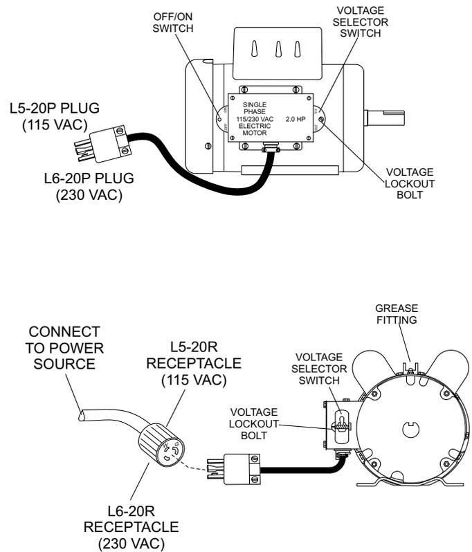
**Figure 12. Single Phase Electric Motor With 12-inch Pigtail**
