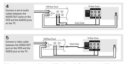
Follow the instructions in "Viewing a VCR or Camcorder Tape" to view your VCR tape. *Note: This figure shows the Standard connector-jack panel. The actual configuration for your TV may be different.*
