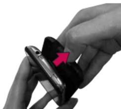
1. Hold the phone with both hands and use the fingertip cutout at the top of the phone to pull open the battery cover (as shown above).
