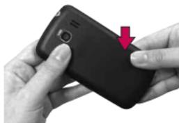
3. Replace the battery cover over the back of the phone (as demonstrated). Apply a steady downward pressure until the battery cover clicks into place.
