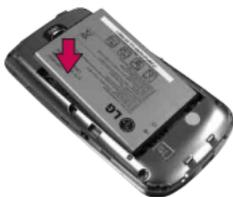
2. Align the battery contacts with the terminals near the bottom of the phone, then press the battery into place.
