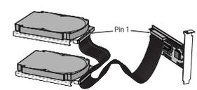
**Caution.** Make sure to align pin 1 on the computer or host adapter interface connector with pin 1 on your drive or drives. Pin 1 on the interface cable is usually indicated by a stripe along the edge of the cable.
