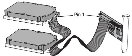
**Caution.** Make sure to align pin 1 on the computer or host adapter interface connector with pin 1 on your drive or drives. Pin 1 on the interface cable is usually indicated by a stripe along the edge of the cable.
