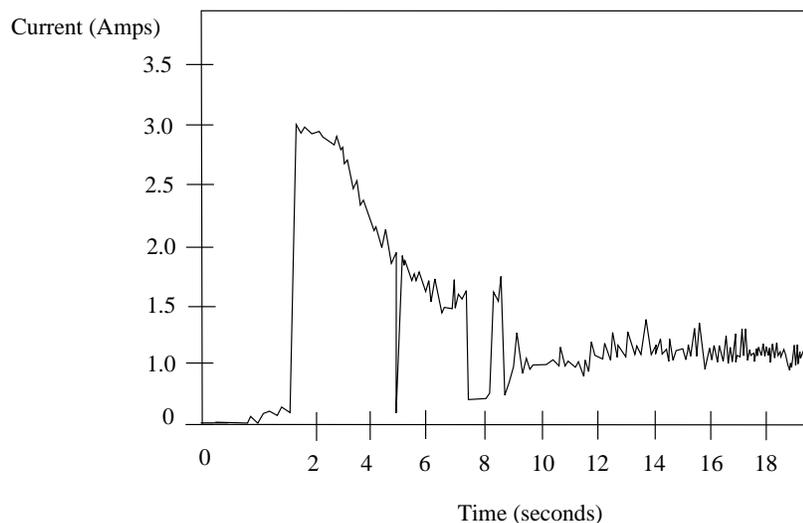
Figure 1. Typical startup current profile
