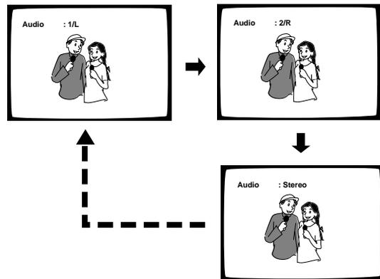
Press **AUDIO** repeatedly during playback to switch the audio type. Audio output changes from "1/L" (Left channel) to "2/R" (Right channel) to "Stereo". This function is possible only in Normal mode.
