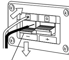
3. Push down the speaker's red tab to open the positive (+) terminal and insert the wire's other conductor. Release the tab.
