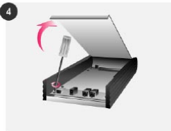
4 Open the top-cover and unscrew the PCB.
