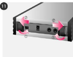
11 Push each hasp to the arrow direction.
