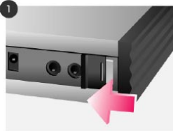
1 Pull a hasp to the arrow direction.
