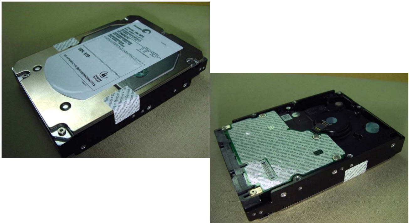
Figure 8. Example of FIPS tamper evidence labels.
