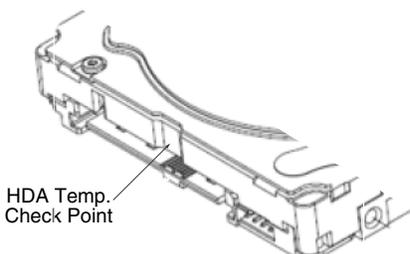
**Figure 7. Location of the HDA temperature check point**
