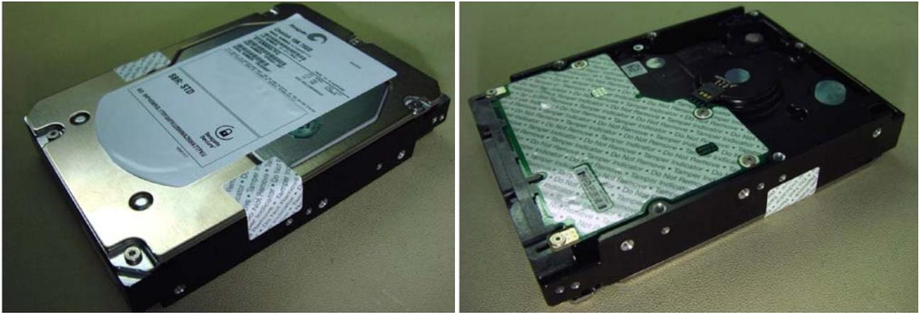
**Figure 10. Example of FIPS tamper evidence labels.**
