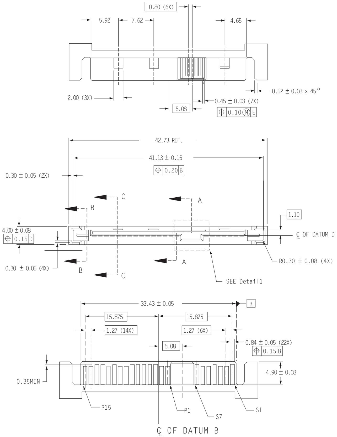
**Figure 14. SAS device plug dimensions**
