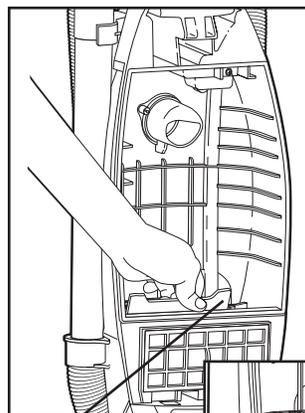
**NOTE:** Frequent cleaning of the filters will maintain maximum efficiency of your cleaner. The foam and pleated filters should be removed for frequent washing and can be used in rotation with extra filters (available through Electrolux Helpline) to ensure clean, dry filters are always ready for use.
