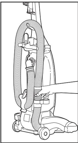
1. To use accessories remove hose from hose retainer on back of cleaner by lifting up and twisting.
