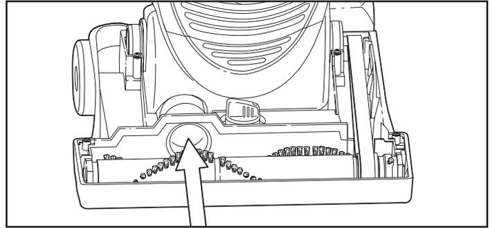
3. Remove the hood from the cleaner and check for a blockage in the brushroll area. Make sure the hose inlet is clear. **If no blockage is found, continue to step 4.**
