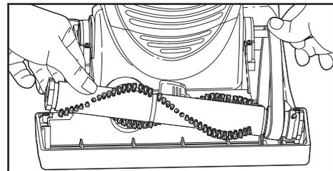
8. Align left end cap with base. Push end cap securely into place.
