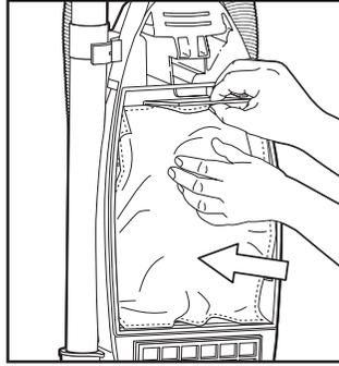
Make sure dirt inlet goes completely into dustbag and bag is pushed completely back into place. Tuck excess bag into cleaner.
