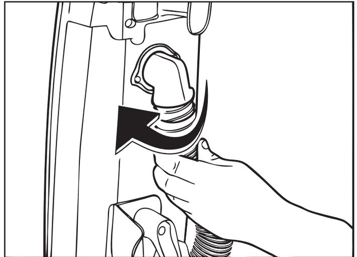
4. Twist the hose from the coupling elbow on the back of cleaner. Check for blockages at cleaner opening and in hose. If a blockage is found, clear the blockage.
