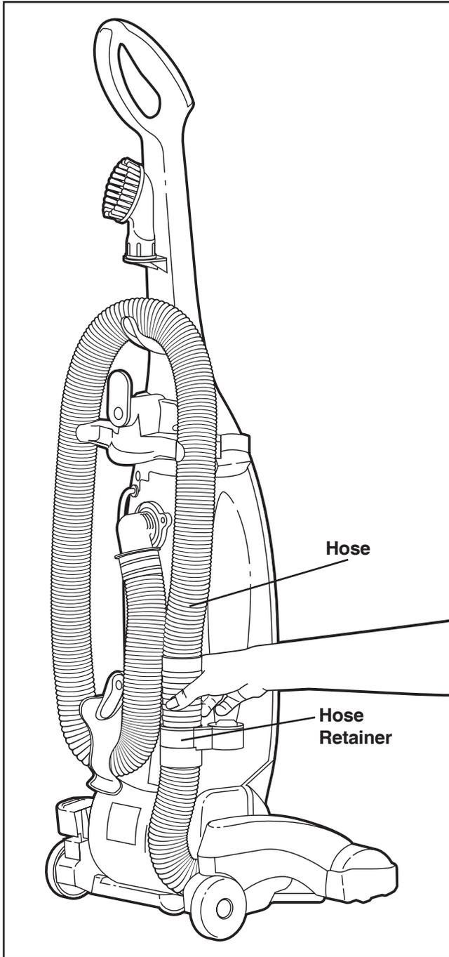
1. Firmly pull the end of the hose from the hose retainer on the back of the vacuum.
