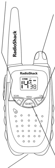
**VOLUME ON/OFF** – Rotate to turn the radio on and off and adjust the volume.
