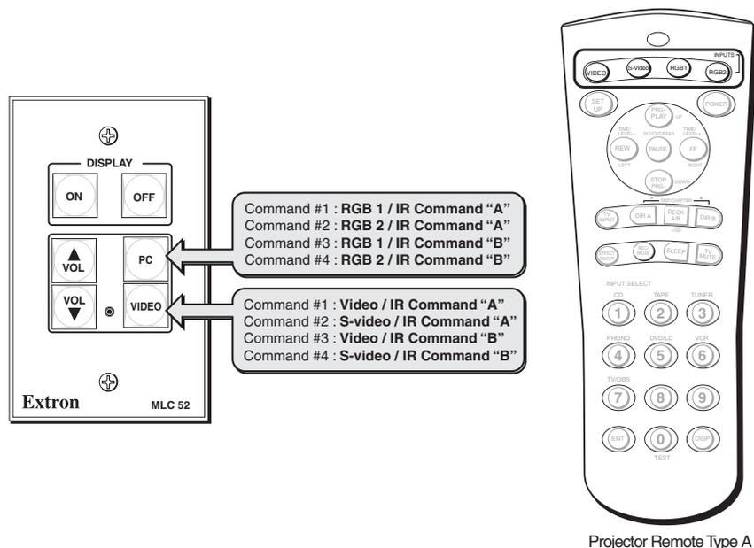
**Programming MLC 52 input selection buttons from a projector remote control type A**
