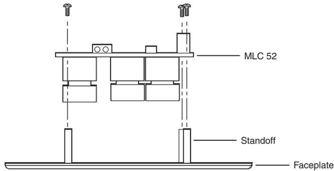
**Installing the MLC onto a new faceplate (bottom view)**
