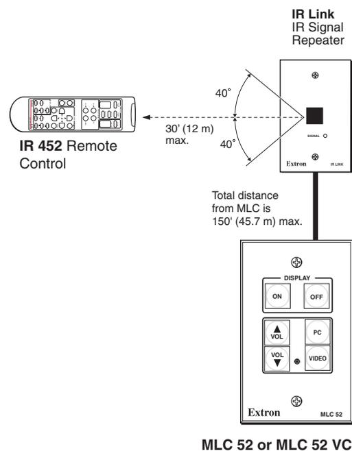
**Using the IR Link with the MLC 52 and the IR 452**
