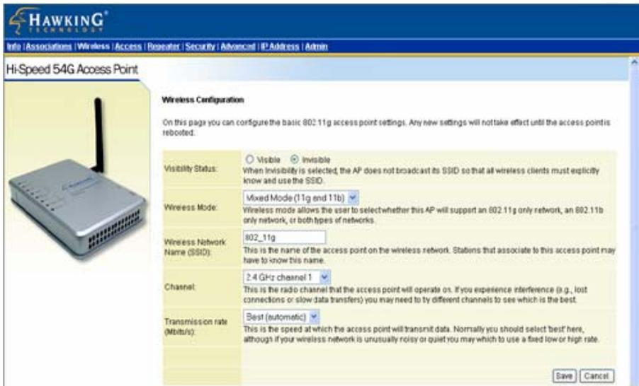
The screenshot shows the configuration interface for a Hawking Hi-Speed 54G Access Point. On the left is an image of the device. The main area is titled "Wireless Configuration" and contains the following settings:
