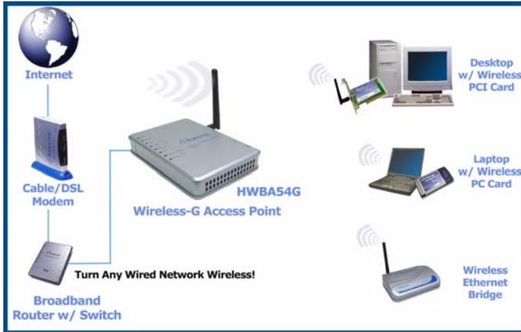
2. **Bridge:** When acting as a Bridge, the HWBA54G serves as a wireless adapter that connects a wired network with another wired or wireless network through an access point(s). See the sample application below.
