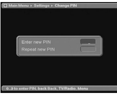
Change of PIN code (standard code = 0000)
