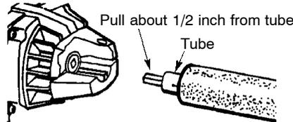
**NOTE:** The end of the drive shaft is square. This square end fits inside a square hole in a shaft inside the engine. Look inside the end of the engine and you will see the square hole in the shaft.
