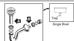
Connect drain assembly hand tight to check alignment. It may be necessary to cut off part of the tailpiece (area "A") or part of the horizontal leg of the trap (area "B").
