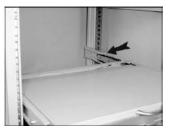
4. Fasten the assembled drawer onto the front brackets using the four screws provided.
