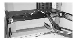
10. Make sure the C-36 connectors are firmly connected:
