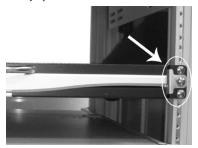
Slide the assembled drawer into the rack cabinet from the front and insert the two slide rails of the assembled drawer into the pockets of the rear brackets.
