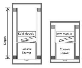
The KVM Module can be connected to a console, or be used as a stand-alone KVM Switch. There are three major categories: PS/2, USB and Sun Interfaces:
