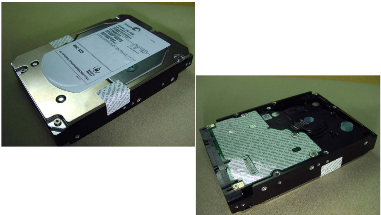
Figure 13. Example of FIPS tamper evidence labels. Does not represent actual drive.
