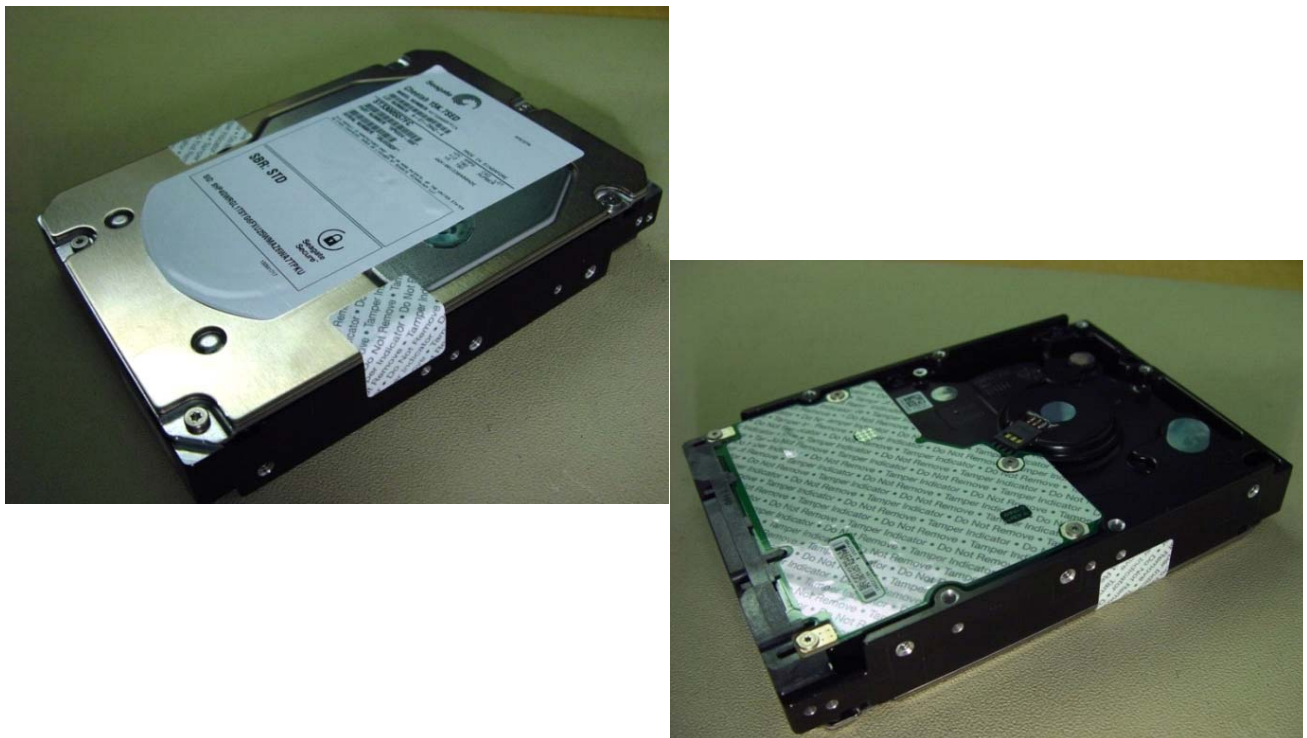
Figure 7. Example of FIPS tamper evidence labels. Does not represent actual drive.
