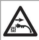
Switch off! Remove plug from mains before adjusting, cleaning or if cable is entangled or damaged.
