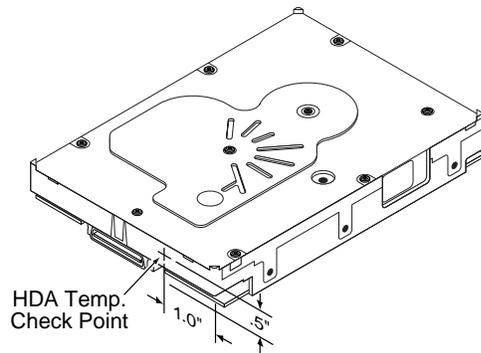
**Figure 10. Locations of the HDA temperature check point**
