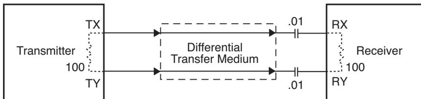
**Figure 17. FC-AL transmitters and receivers**
