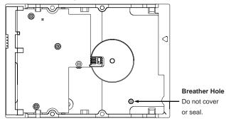
Caution. Do not cover, seal, or insert any object into this hole.
