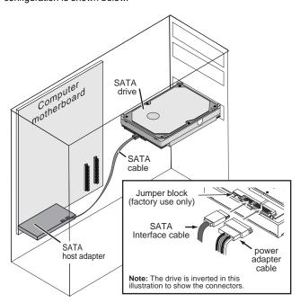
Note. Serial ATA connectors are keyed to ensure correct orientation.
