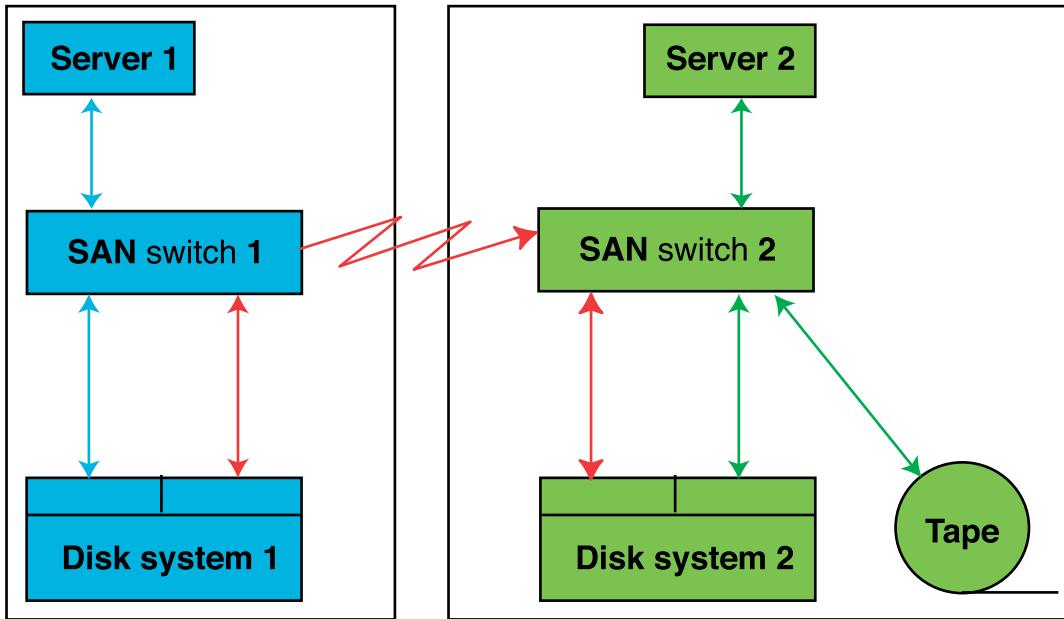
Many disk subsystems, including IBM TotalStorage DS4000 series, are capable of copying data to a remote location. The data path for the remote copy operation is represented by the red links in the diagram.
