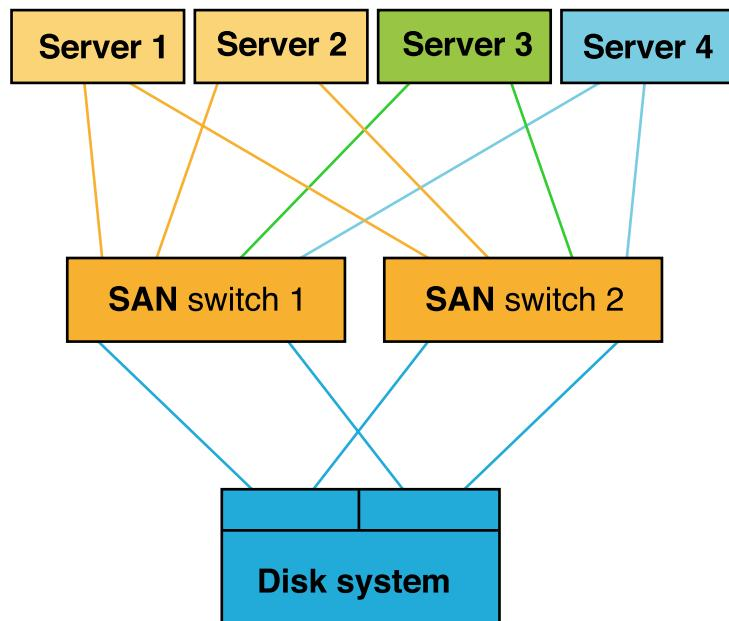
redundant Host Bus Adapters. And each Host Bus Adapter is connected to a different SAN switch, and each switch is connected to a different controller in a disk system. Every effort is made to provide continuous application access to data.
