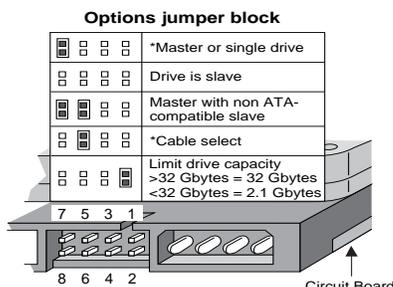
Refer to the jumper settings on your drive label to configure the drive for your system. Jumper settings also can be accessed online from our Web site at [www.seagate.com](http://www.seagate.com).
