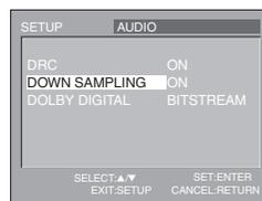
**ON** : When outputting in 48kHz.
