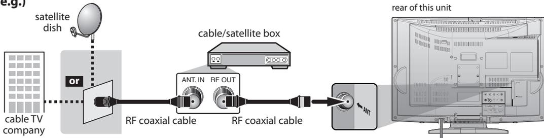
\*Required cables and connecting methods differ depending on the cable/satellite box.
