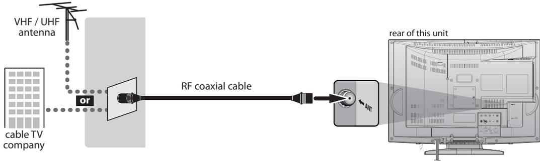
\*Once connections are completed, turn on the unit and begin initial setup.
