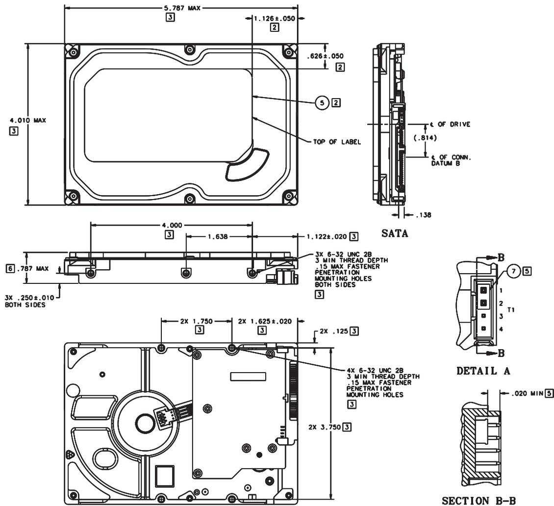
Figure 3. Mounting dimensions
