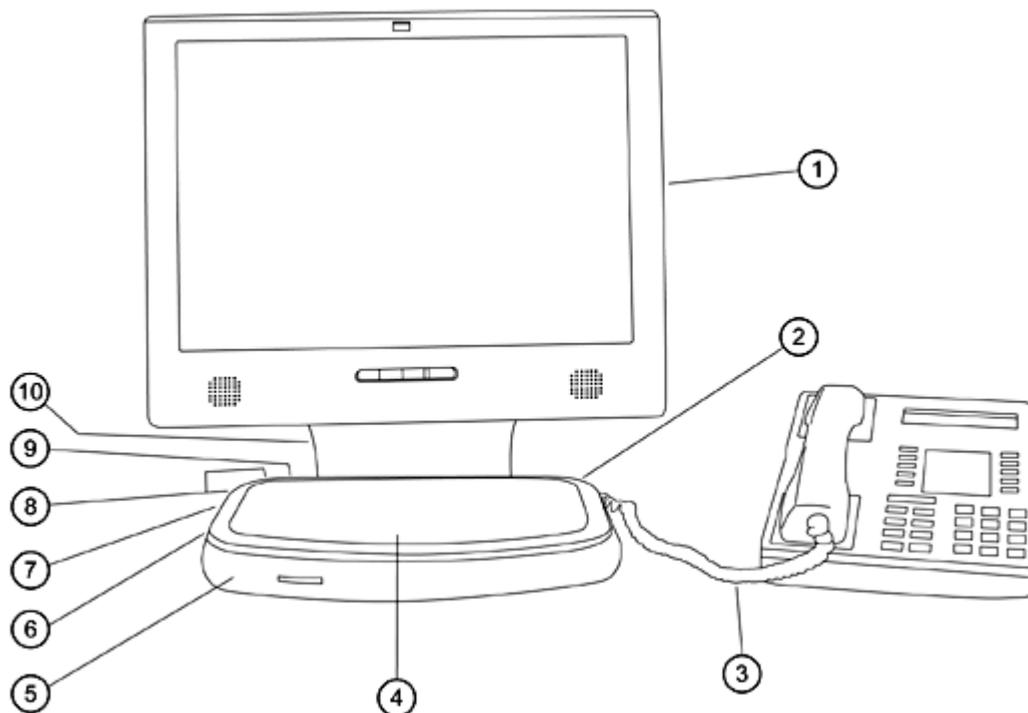
1. Display purchased separately. Desktop Access center integrates into the base of the L1530 and L1730 monitors which can rotate into portrait orientation. The Desktop Access center complements other HP monitors.
