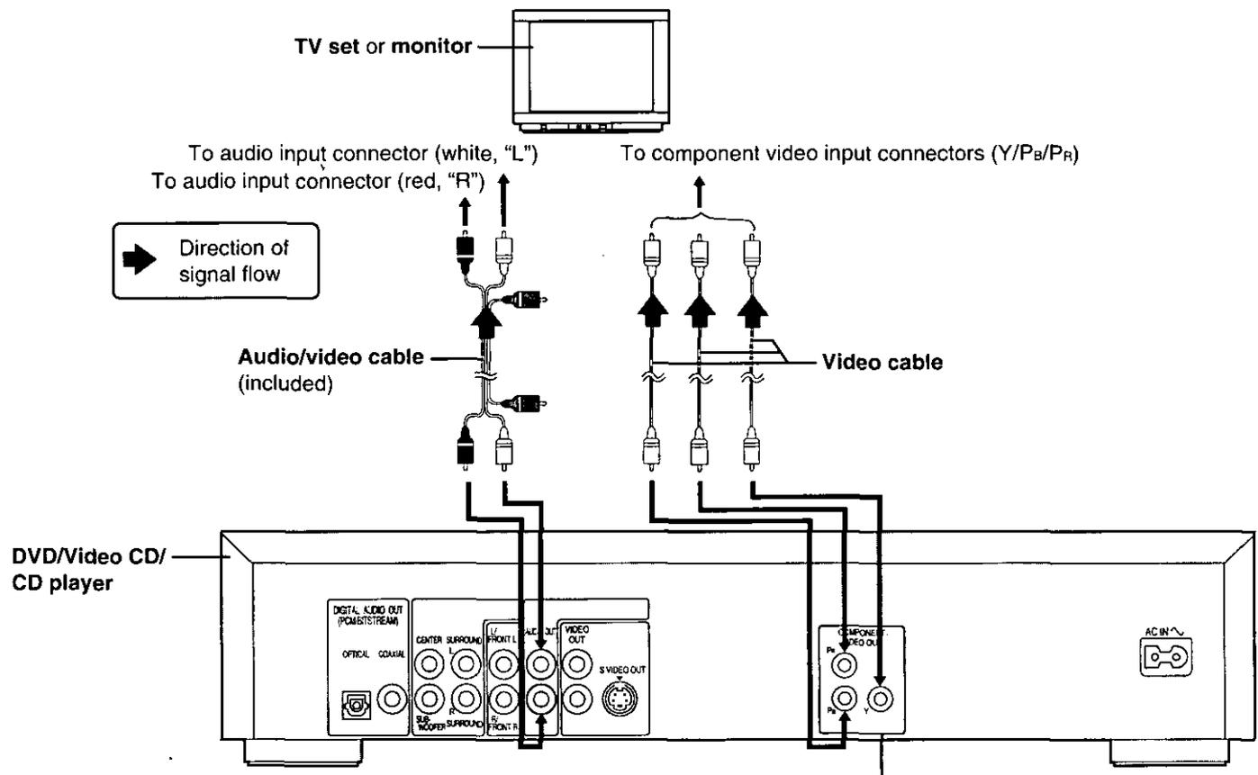
**Component video output connectors (Y/P<sub>B</sub>/P<sub>R</sub>)**
