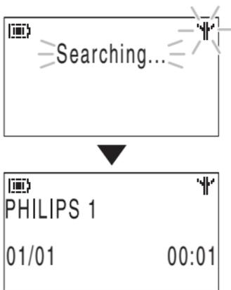
The display will show the word “Searching” and Antenna icon flashing until it locks onto its subscribed. Then the display shows the standby display.
