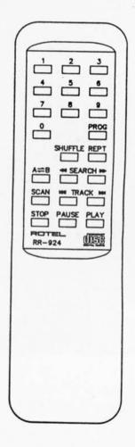
The A-B button will create a "time loop" in the music. Press the button once, when you reach the *start point* (time) of the loop in the music. Press it a second time to select the *end point* (time) of the loop. Pressing STOP or the A to B button a third time defeats this feature. The A to B feature will be useful if you wish to learn the words or the chords to a song. A-B will appear in the display.
