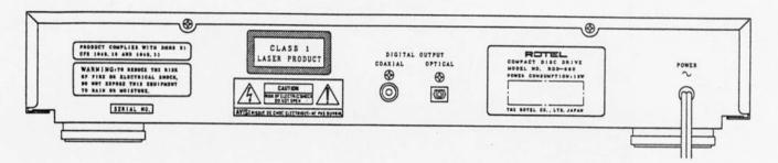
Please refer to this drawing of the Rear Panel of the RDD 980 when connecting to your Digital to Analog Converter.
