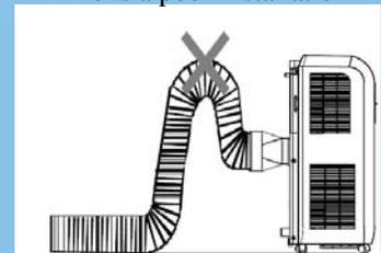
When installing the exhaust hose, try and keep it as flat as possible. The less angles and bends in the hose, the better the unit will perform. If bending or an angle is necessary, use single 90° angles like the pictures above. Multiple bends will decrease performance and efficiency
