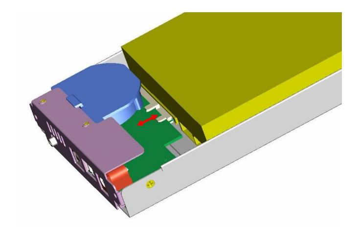
Push the HDD toward the PCB and make sure the connector is well connected.
