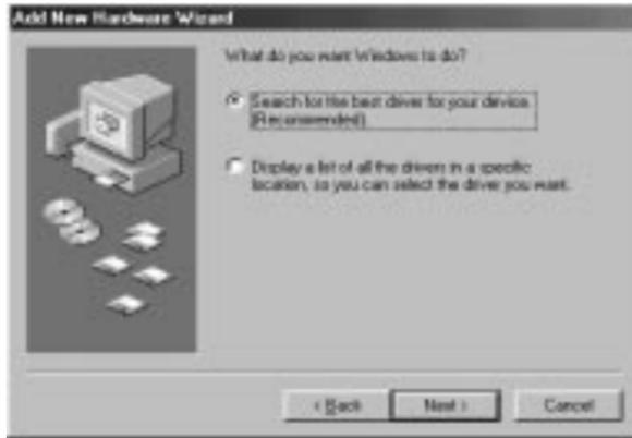
8. When the following window appears, check the **Floppy disk drives** box. Then insert the support software floppy disk into the floppy disk drive and click on the **Next** button.
