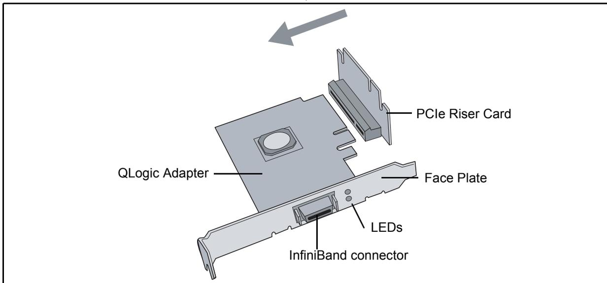
**Figure 4-5. QLogic PCIe HCA Assembly with Riser Card**
