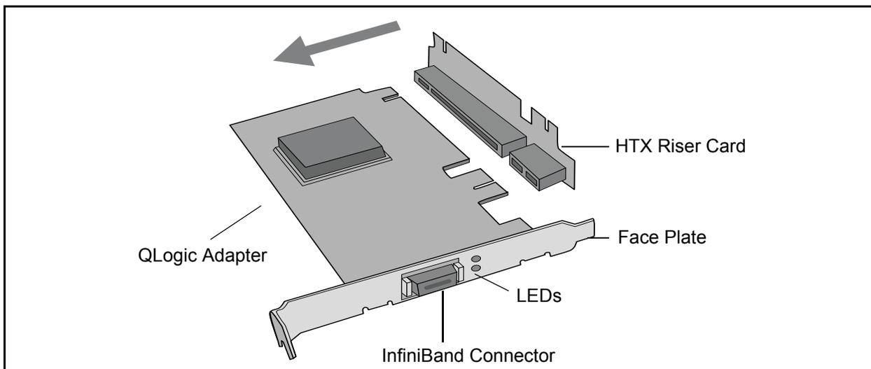
**Figure 4-8. QLogic QHT7140 Adapter with Riser Card**
