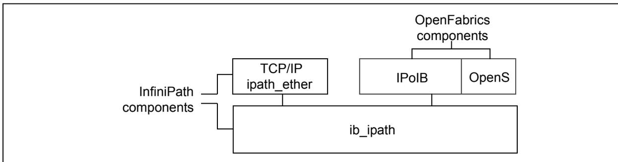
**Figure 5-1. Relationship Between InfiniPath and OpenFabrics Software**
