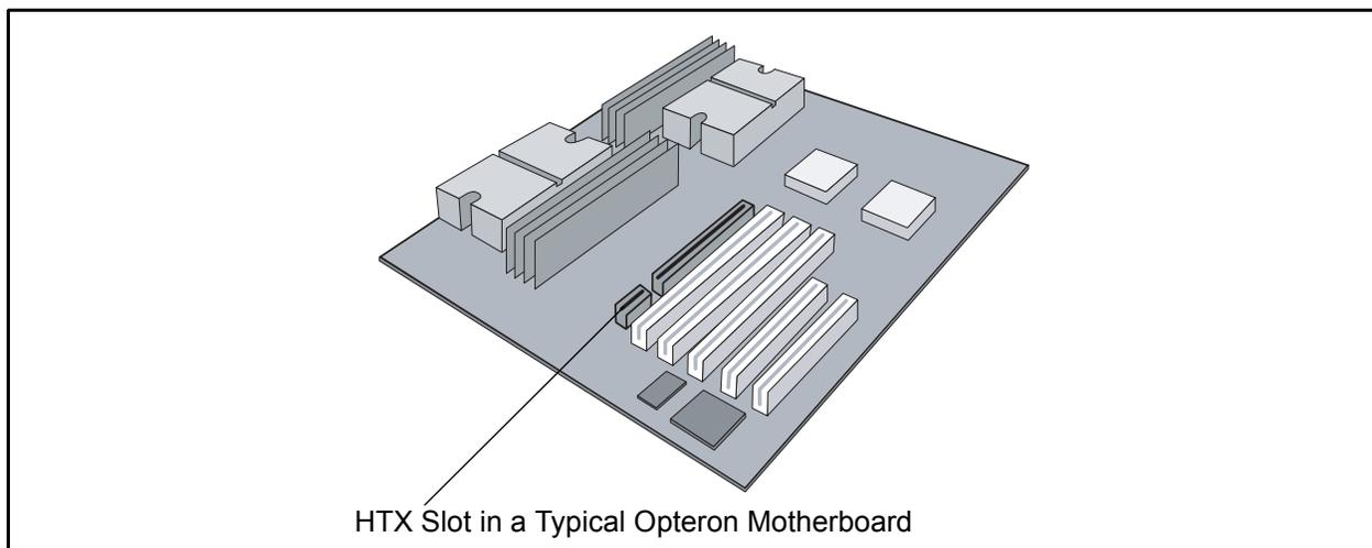
**Figure 4-7. HTX Slot**
