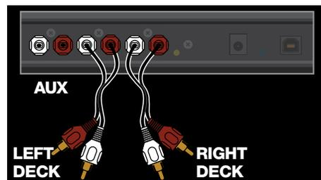
Connect the OUTPUTS of the SL 3 to line inputs on your mixer. Connect the AUX output to an additional line input or AUX input on your mixer to output the sample player. SEE "SAMPLE PLAYER" ON PAGE 18.
