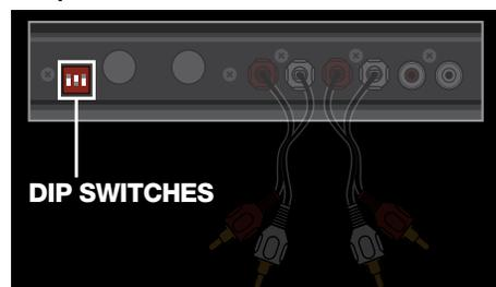
Set each input to the correct input level using the dip switches. Set the switches UP for Phono (turntables) or DOWN for Line (CD players).
