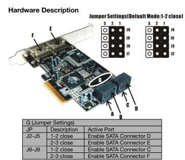
**Note:** There are six SATA ports in PCle SATA II 300 4-Channel Adapter. We name these ports A to F. Ports A to D are internal SATA ports and E & F are external SATA ports. By changing the jumper setting on the PCle SATA II 300 4-Channel Adapter that allows you to select between external and internal ports to use.. By default, Port A, B, C and D are working.
