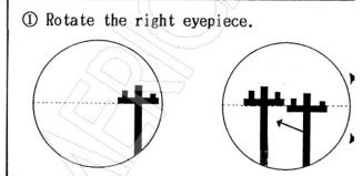
② If it is not possible to level it with the image of the left eyepiece by rotating the right eyepiece, try to do the same adjustment as the above by rotating the left eyepiece.
