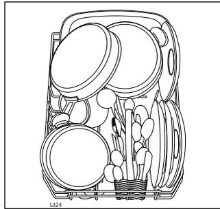
The two rear rows of prongs on the lower basket can be easily lowered to allow you to load pots, pans and bowls.
