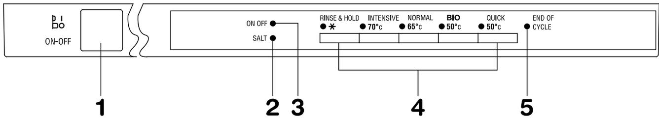
In this fully integrated appliance the controls are located on the top of the door. When selecting a programme, the door needs to be open.
