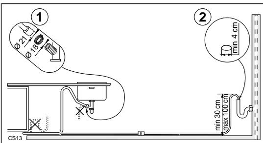
The waste connection must be at a height of between 30 cm (minimum) and 100 cm (maximum) from the bottom of the dishwasher.
