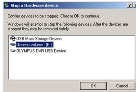
Clicking on the [Stop] button launches another dialog box to confirm the devices that are to be stopped. Clicking the [OK] button closes the USB connection.
