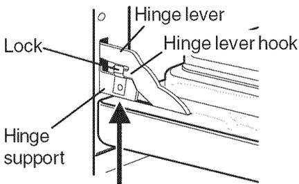
Lock engaged for door removal
