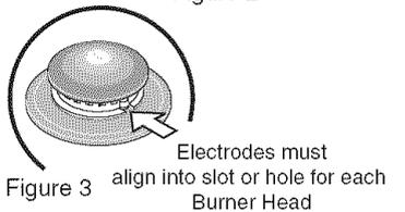
**REMEMBER — DO NOT ALLOW SPILLS, FOOD, CLEANING AGENTS OR ANY OTHER MATERIAL TO ENTER THE GAS ORIFICE HOLDER OPENING.** Always keep the Burner Caps and Burner Heads in place whenever the surface burners are in use.
