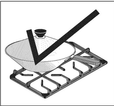
**Woks** with flat bottoms suitable for use on your cooktop are available in most cookshop or hardware stores. Round-bottomed woks (with a support ring that does not extend beyond the burner circumference) may also be used. The metal ring was designed to support the wok safely when it is filled with large amounts of liquids (soup making) or fat (frying).
