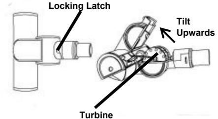
1. Slide locking latch forward then tilt the top housing of the brush upwards. The top housing is hinged and will tilt up approximately 45° only.
