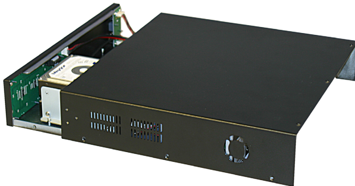
Figure 5. Removing the Top Cover
