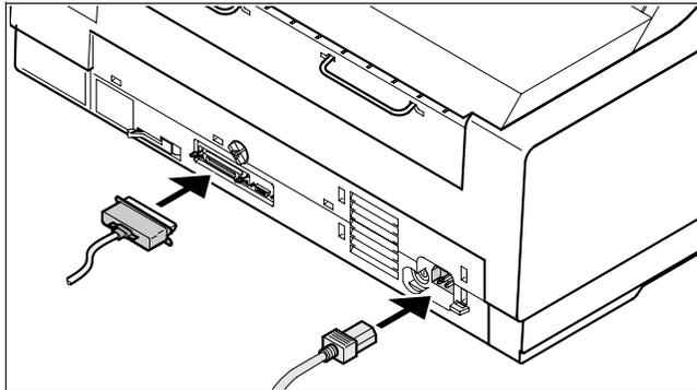
Make sure that the printer and the computer are switched off, and connect the printer to the computer with the data cable (interface cable).
