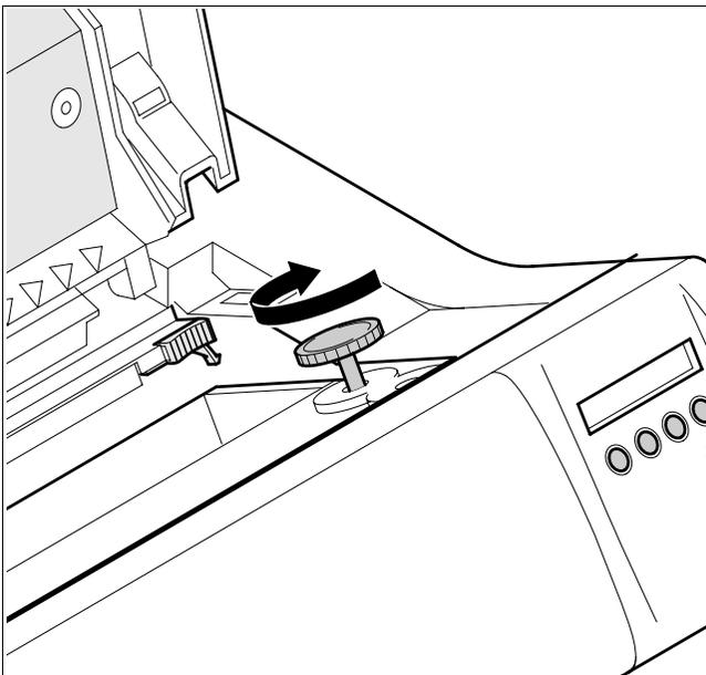
Insert the coloured tension knob into one of the two locations. Turn the tension knob to take up slack in the ribbon until it is seated correctly at the bottom in the ribbon support.
