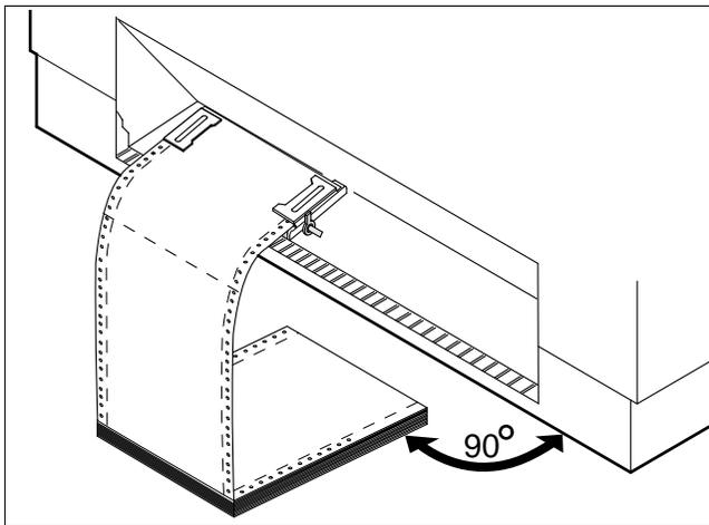
Be sure to align the paper stack in parallel with the printer and that the paper flow is unobstructed.
