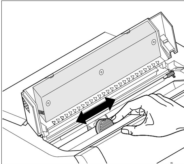
Move the print head carriage backwards and forwards several times. If the ribbon is correctly seated, there must be no perceptible resistance.
