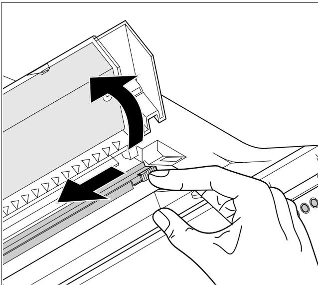
Move the coloured friction tab to the left (direction of the arrow) as shown in the figure and raise the friction mechanism.
