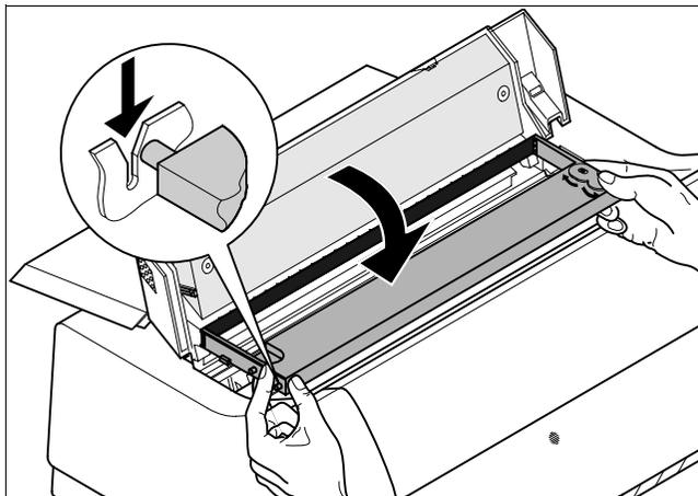
Tilt the ribbon cassette slightly forward, and thread in the ribbon between the coloured insertion tongue and the ribbon support (transparent plastic plate). Align the cassette and insert it, then press down until it clicks into place.
