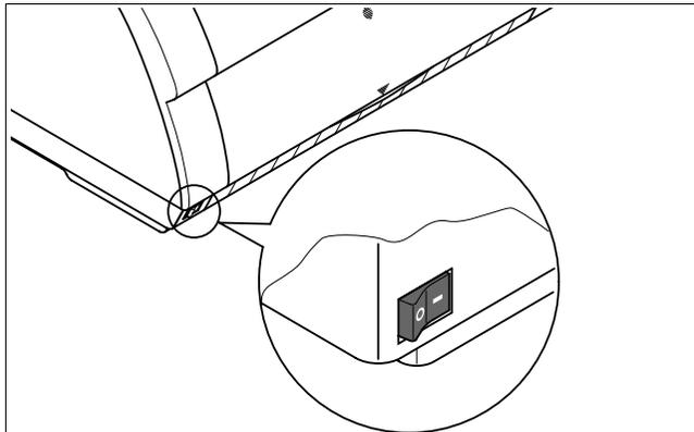
The power switch for switching on the printer is located at the bottom left at the front of the printer when viewed from the front.
