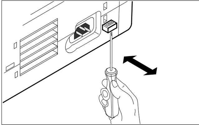
Make sure that the printer is set to the correct voltage (e.g. 230 V in Europe, 120 V in the U.S.A.). To do this, check the plate above the power inlet at the rear of the printer. If the setting is incorrect, set the coloured switch at the rear of the printer to the correct position, using a pointed object (e.g. screwdriver, ball pen or tweezers).
