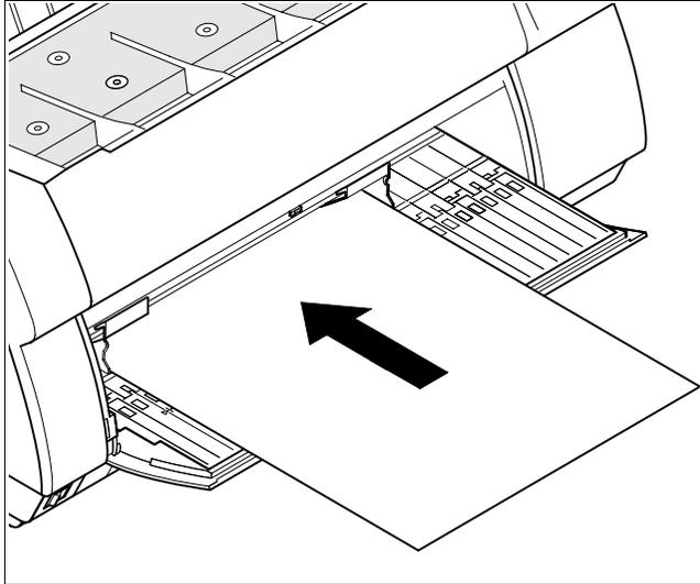
Insert the single sheet as far into the input tray as possible. Press the **Online** key to set the printer to ready status. The sheet is automatically loaded when the printer is in online mode and receives data from the computer. Press the **Load** (4) key to load paper before starting the printout.
