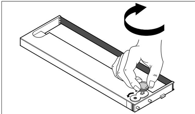
Insert the coloured ribbon tension knob into the right-hand front location of the new ribbon cassette. Turn the knob in the direction of the arrow in order to take up the slack of the ribbon.
