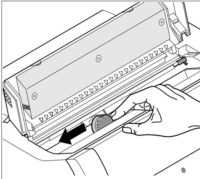
Carefully slide the print head carriage to the left stop (viewed from the printer front).
