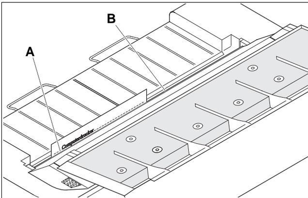
The paper is fed to the position where the bottom edge of the first printing line **A** is aligned with the tear edge of the top cover **B**. The factory setting for the first printing position (TOF) is 12/72".
