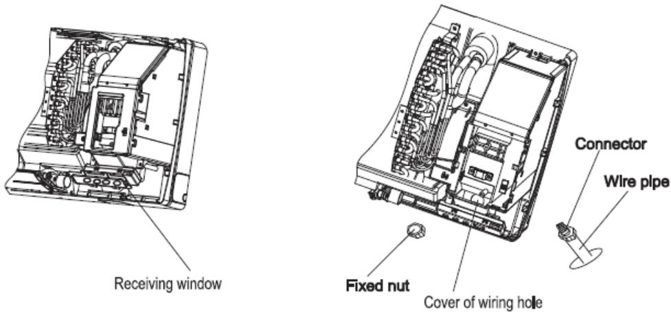
4. Wire pipe should be tightened by the fixed nut and the electric box should be fixed as shown in the above right figure and the below figure.
