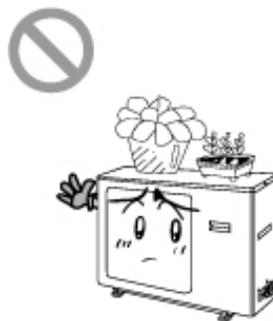
★ Don't block the air intake or outlet vents of both the outdoor and indoor unit. It can decrease the air conditioning capacity or cause a malfunction.
