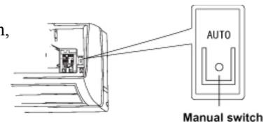
Turn on the unit: By pressing the Manual Switch the unit will start in AUTO automatically. The microcomputer will adjust to the indoor temperature by selecting (COOL, HEAT, FAN), in order to achieve a comfortable condition.
