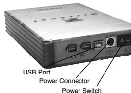
**Note:** in order to reach USB 2.0 speeds, you must have a computer or host adapter that has USB 2.0 support. Your MicroNet storage device will autosense the highest available connection speed.
