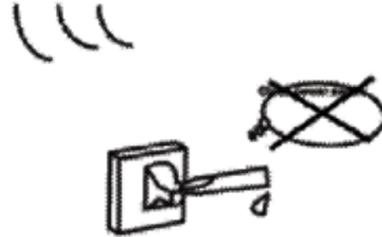
★ Don't touch the metal part of indoor unit after taking out the filter. It will cause an electric shock.
