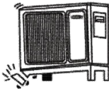
★ Don't step on the top of the outdoor unit. As falling off the outdoor unit can be dangerous.
