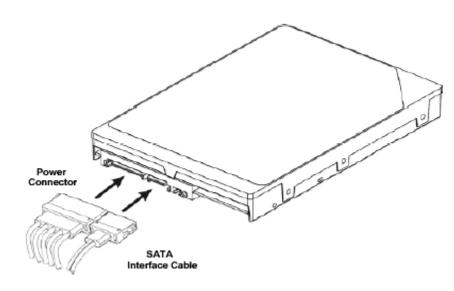
PLEASE NOTE: Unlike standard ATA drives, Serial ATA drives DO NOT require the use of jumpers to configure the drive. Please disregard any references to jumper settings and Master, Slave and Cable Select configurations in the Maxtor Installation Guide.
