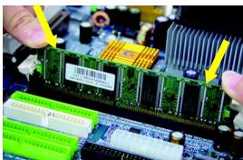
2. Insert the DIMM memory module vertically into the DIMM socket. Then push it down.
