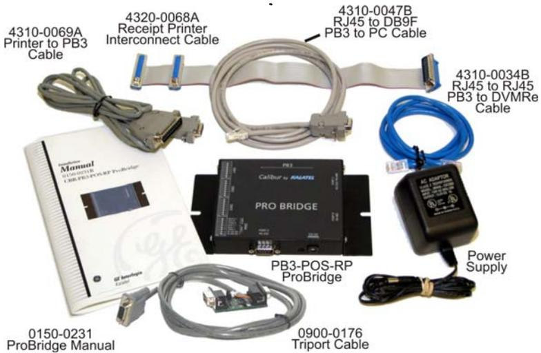
Figure 1-1. PB3-POS-RP Box Contents.
